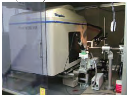
3. Ultra-high brilliant X-ray generator with a high performance imaging plate diffractometer & Free mounting system (FMS)
