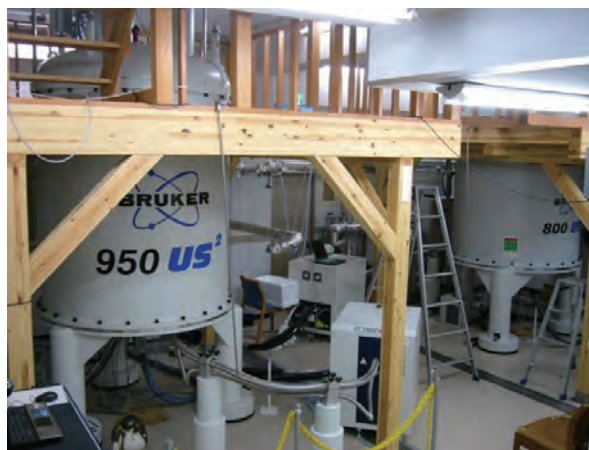
Fig. 1. The 950 and 800MHz NMR machines containing a superconducting magnet and cryogenic probe for each. The sensitivity of the 950MHz NMR reaches about 17-times the value that is exhibited by a normal 400MHz machine. Therefore, the measurement time can be saved by 1/300. The machines are also used for dilute samples within a shorter period, and for isotopically non-labeled samples. The superconducting is maintained by cooling the coil for the static magnetic field down to 2K with liquid helium.
