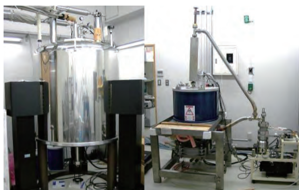
Fig. 1. NMR magnet for 600-MHz solid-state NMR on the left and 395-GHz gyrotron for high-intensity light source of terahertz-wave on the right. Hyperpolarization generated with these instruments increases the NMR sensitivity of proteins. This DNP-NMR spectrometer was developed in Institute for Protein Research. (Ref. 3)
