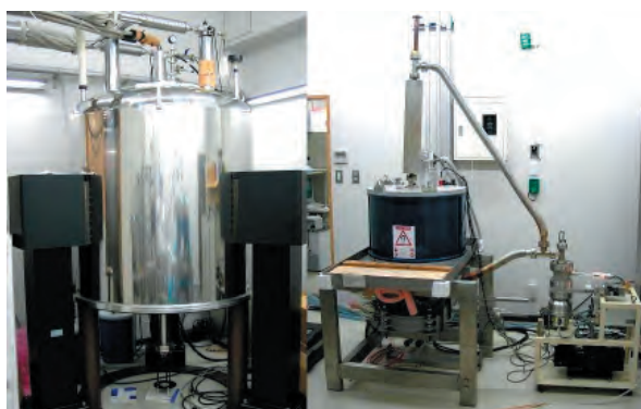
Fig. 1. NMR magnet for 600-MHz solid-state NMR on the left and 395-GHz gyrotron for high-intensity light source of terahertz-wave on the right. Hyperpolarization generated with these instruments increases the NMR sensitivity of proteins. This DNP-NMR spectrometer was developed in Institute for Protein Research. (Ref. 4)
